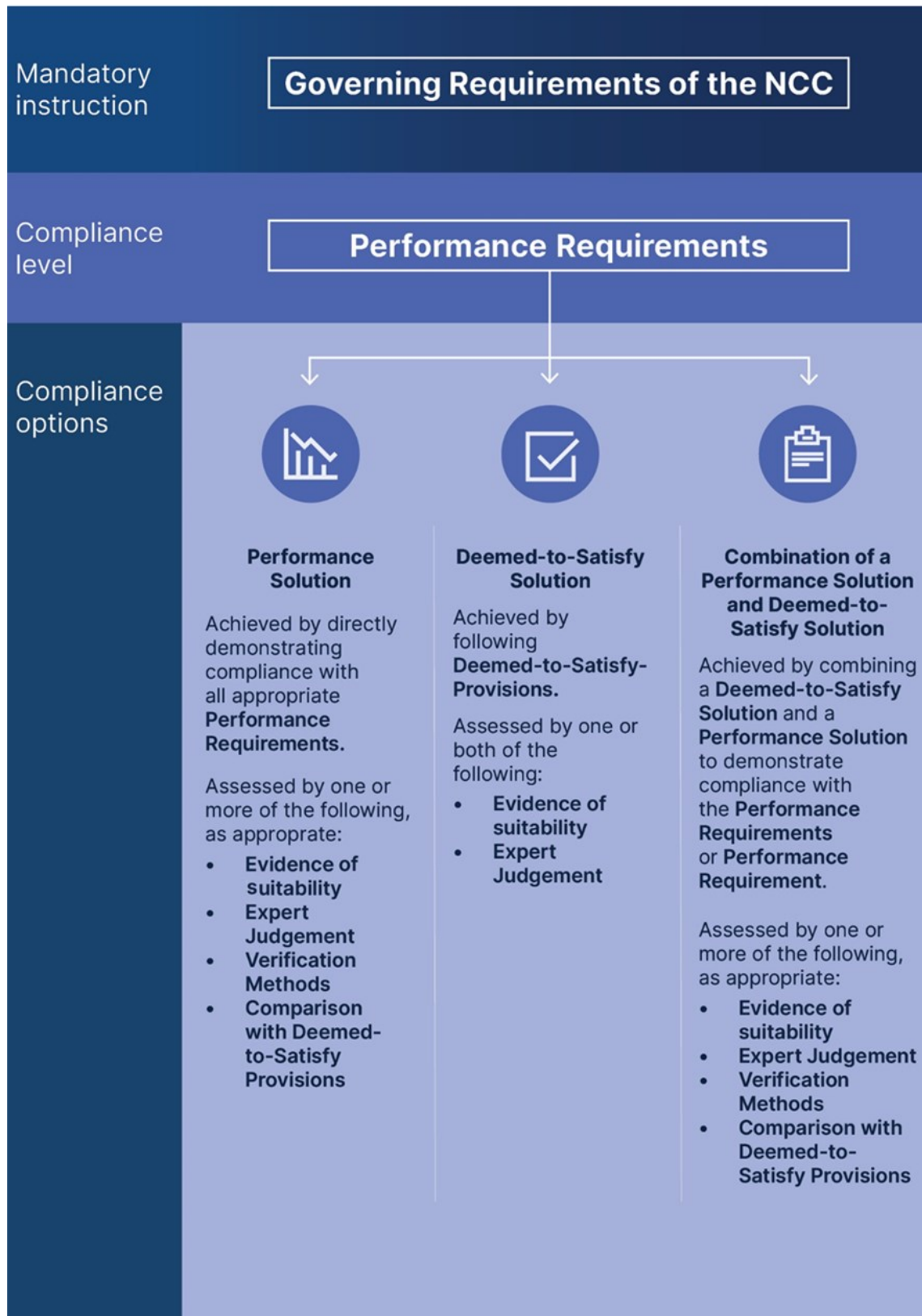
Figure C.1 Demonstrating compliance with the NCC
