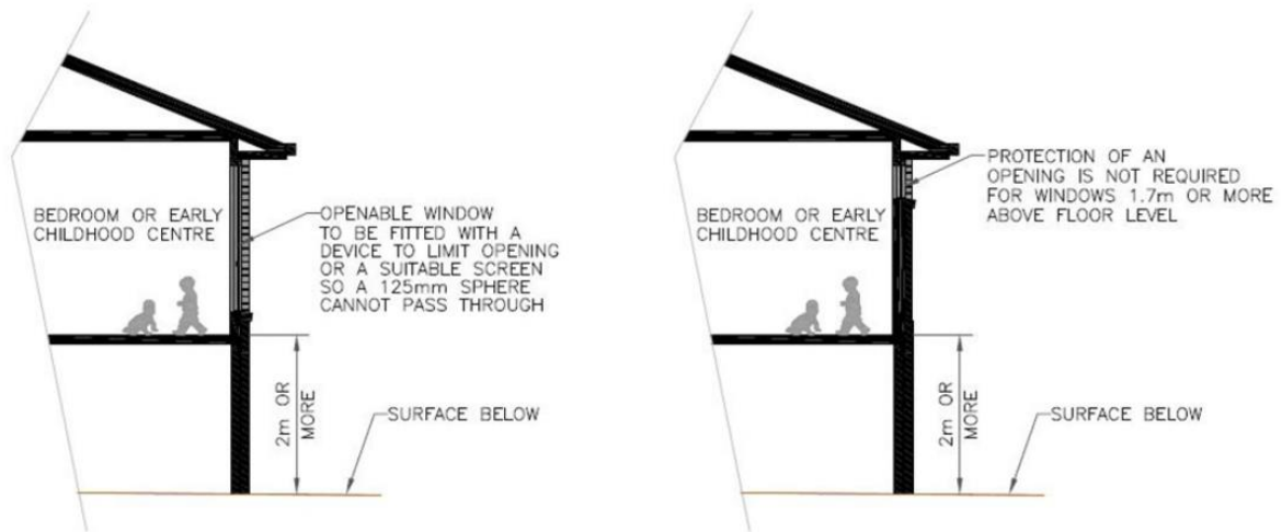
Figure 13 NCC safety provisions for operable windows demonstrating where opening must be restricted to 125mm for safety
