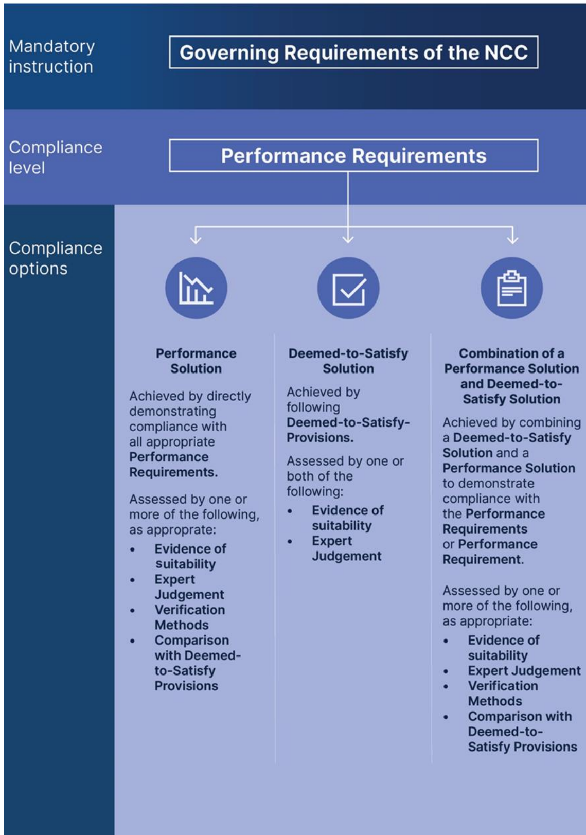
Figure C. 1 Demonstrating compliance with the NCC
