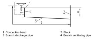
Figure 7 — Limitations for ventilated discharge branches in system I, II and IV
