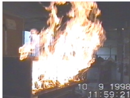
(b) Diagonal view from front left side, some front trays beginning to run low in fuel
