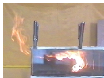
(b) Flames from front of tray 325 mm from vent
