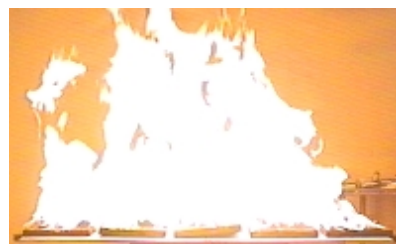
Double Row of Five Trays Per Row - arranged as for 1500 mm by 600 mm enclosure
