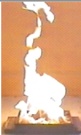
Figure 3 Burning of Single Tray in Open
