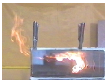
(b) Flames from front of rear tray after fuel in front tray exhausted - flames largely from front edge of tray, curve upward then towards vent (note obscuration of flames near vent due soot deposited on glass)
