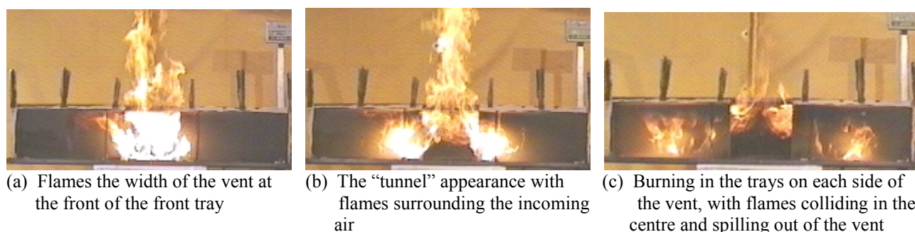
Figure 10 Front Views of Fire in Enclosure 1500 mm Wide, 600 mm Deep and 300 mm High Vent 300 mm wide by 275 mm High
