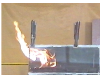
(a) Flames from front of front tray shortly after ignition - flames rise mainly from front edge of tray, travel back and up, and then largely forward and out of the enclosure
