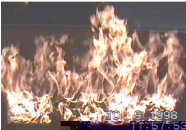
(a) View from directly in front - front trays burning, rear trays not burning
