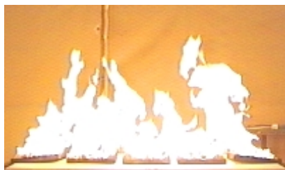
Single Row of Five Trays - arranged as for 1500 mm by 300 mm enclosure
