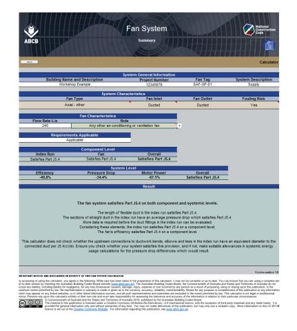
Figure 13.9 Fan System Calculator 'Index Run' page – supply fan
