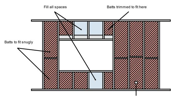
Figure 11.3 Installing bulk insulation in framed walls
