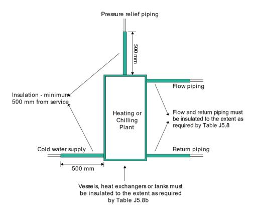
Figure 13.22 Insulation of piping serving a heating or cooling system
