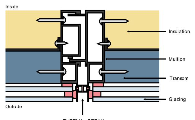
Figure 11.19 Example of a spandrel panel with thermal break
