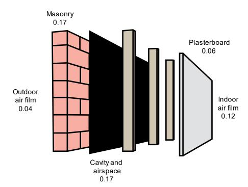
Figure 11.10 Typical wall construction R-Values
