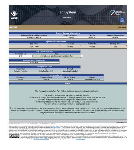
Figure 13.12 Fan System Calculator 'Index Run' page – exhaust fan
