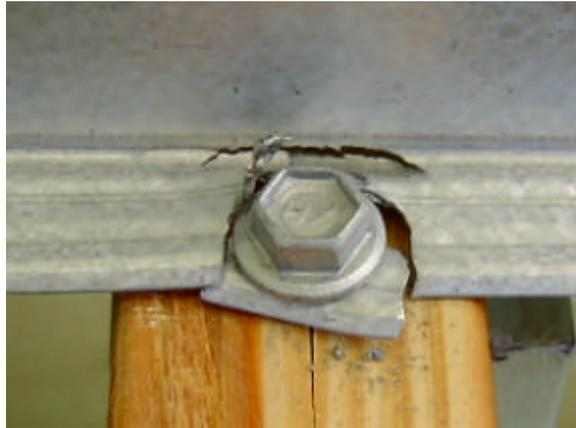
Figure 4.14 Batten failure in Cyclone Testing Station air-box test
