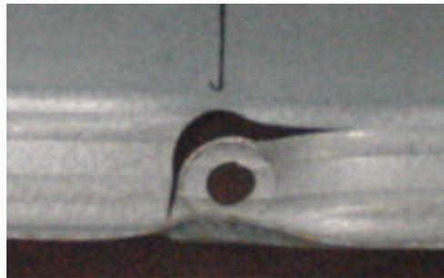
Figure 4.6 Stramit Batten failure mode
