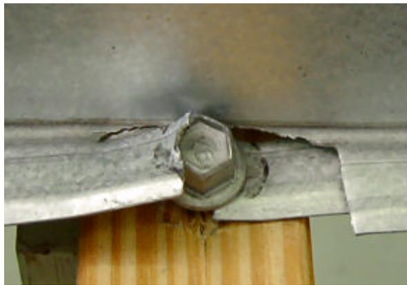
Figure 4.15 Batten failure in Cyclone Testing Station air-box test
