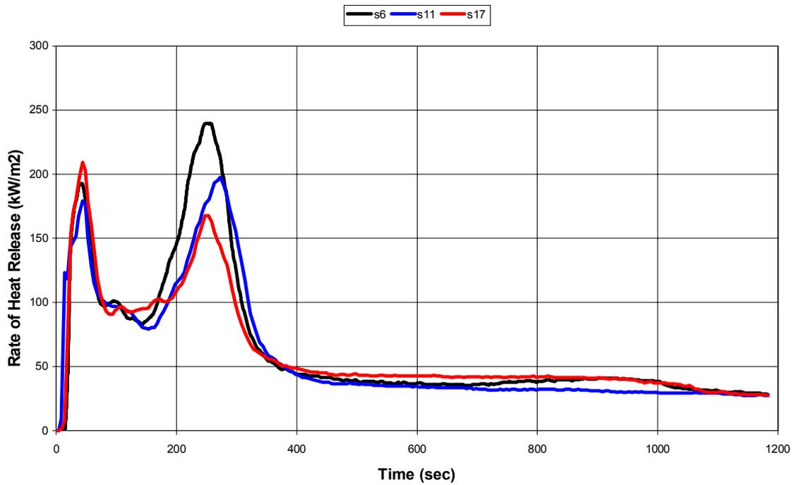
**Figure 6: Heat Release Rate – System A**
