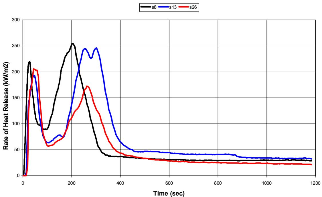
**Figure 7: Heat Release Rate – System B**
