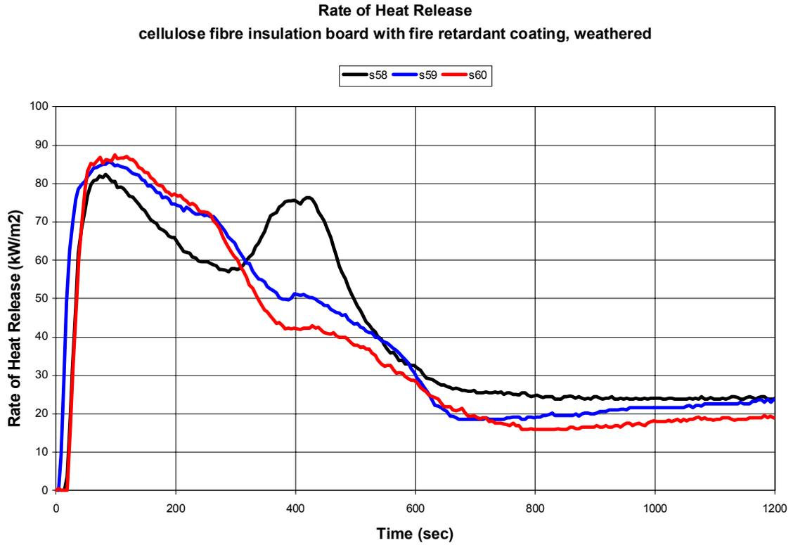
**Figure 18: Heat Release Rate – System M**
