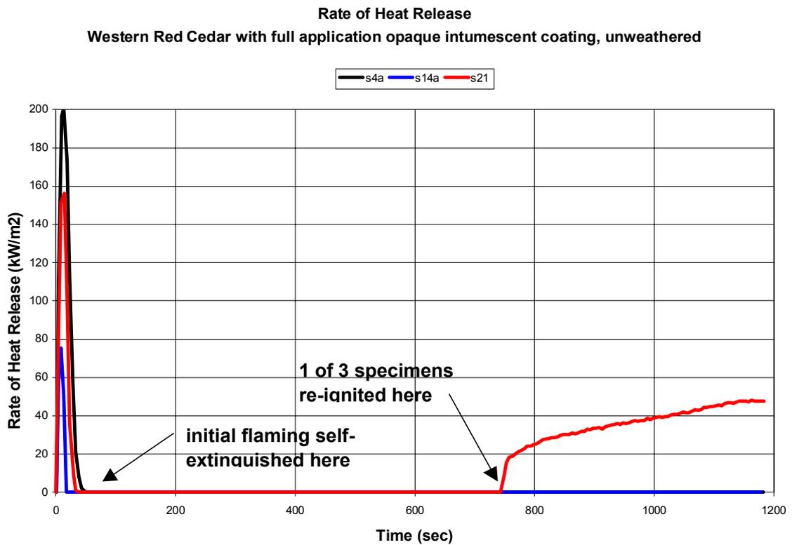
**Figure 23: Heat Release Rate – System R**
