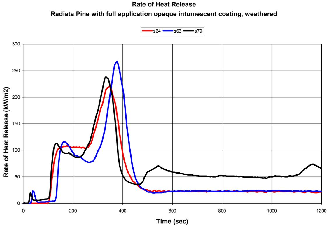
**Figure 10: Heat Release Rate – System E**
