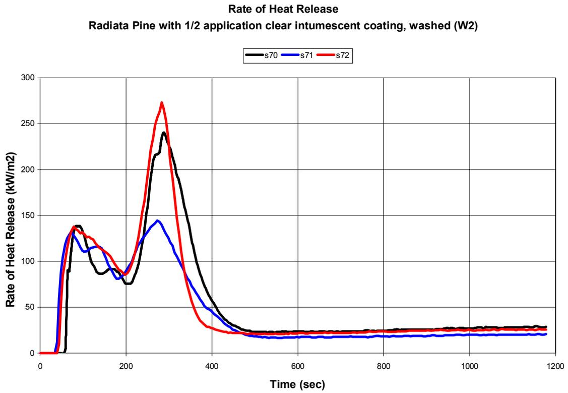
**Figure 16: Heat Release Rate – System K**
