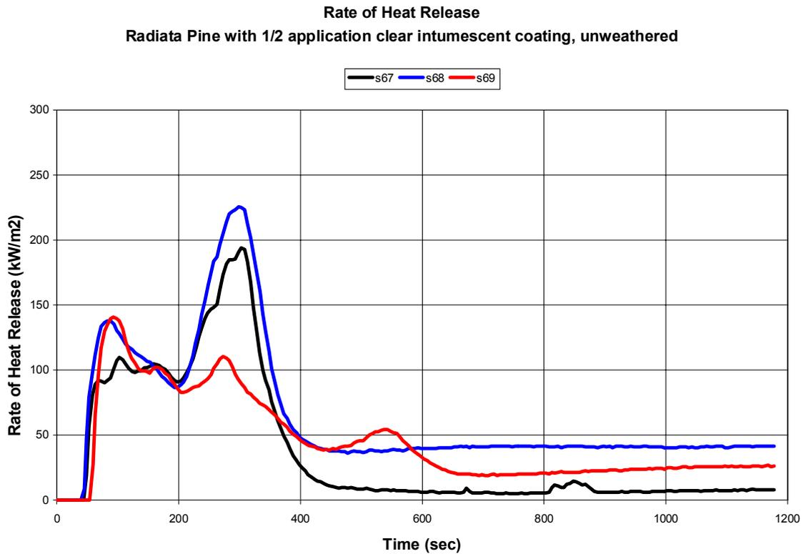
**Figure 11: Heat Release Rate – System H**
