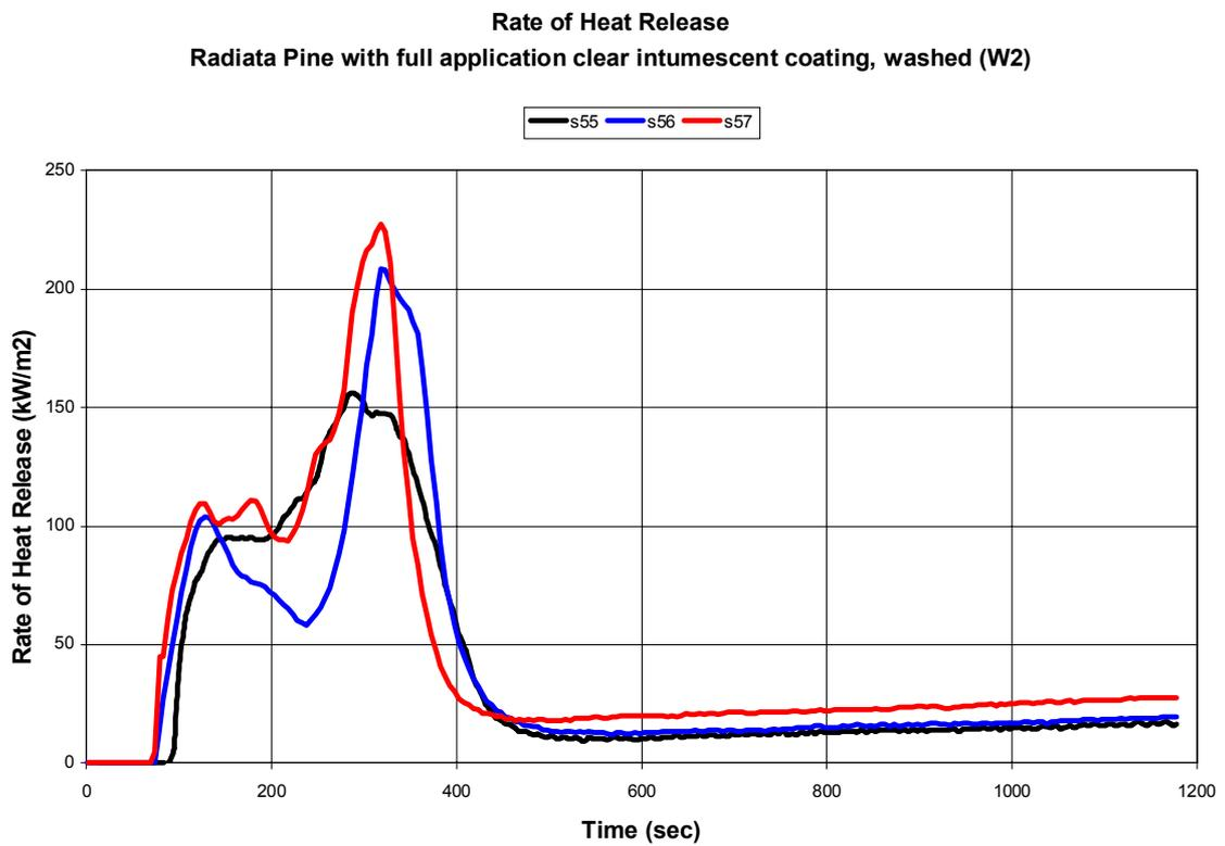
**Figure 15: Heat Release Rate – System J**
