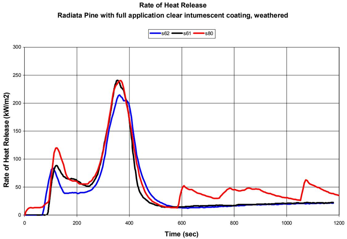
**Figure 14: Heat Release Rate – System G**
