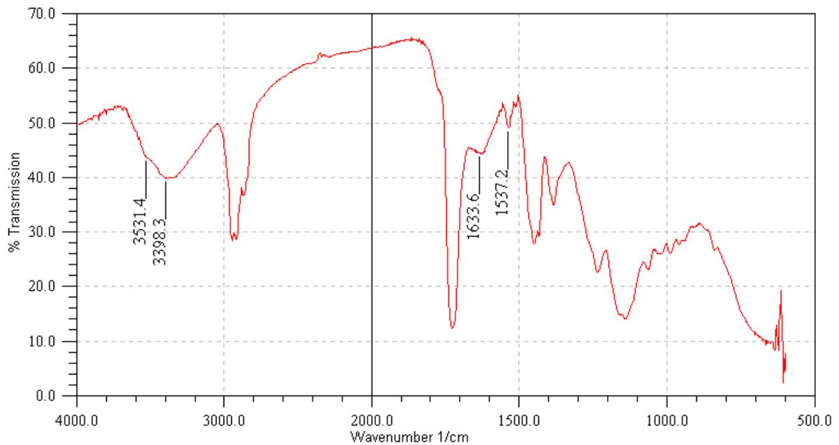
**Figure 4: External Intumescent Coating Topseal After QUV Exposure**
