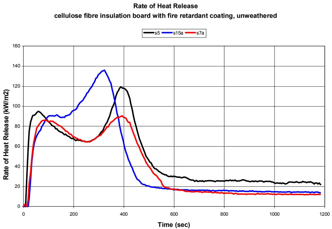
**Figure 17: Heat Release Rate – System L**
