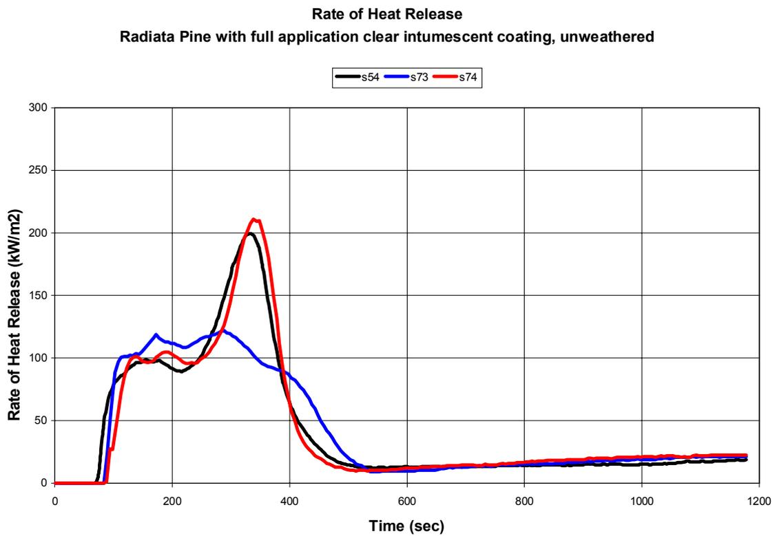
**Figure 13: Heat Release Rate – System F**
