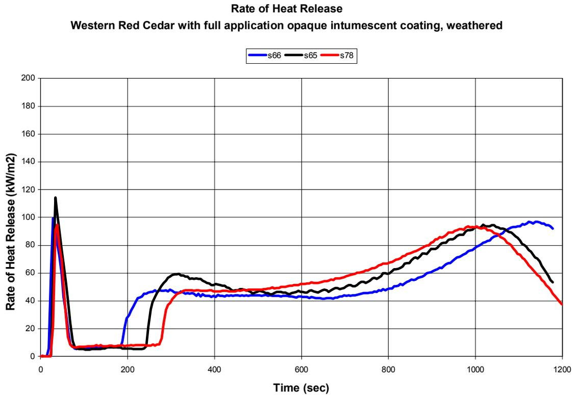
**Figure 24: Heat Release Rate – System Q**
