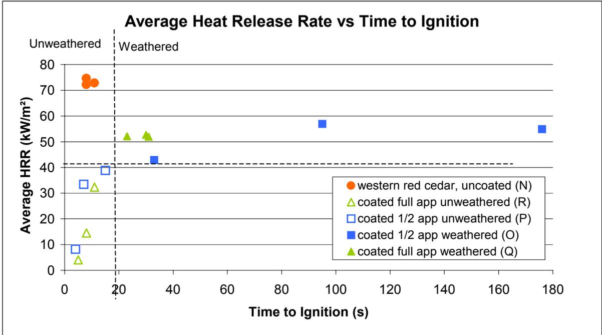
**Figure 29: Comparison of Average RHR and Time to Ignition for the Exterior Western Red Cedar with Opaque Intumescent Coating**
