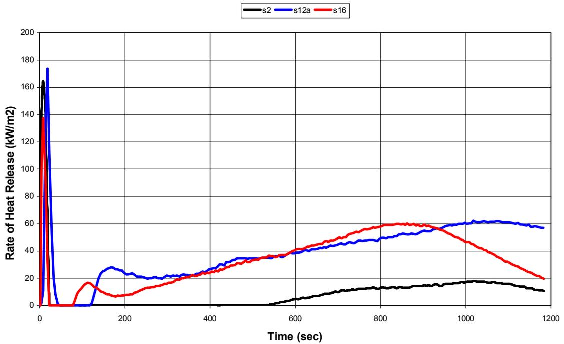
Figure 21: Heat Release Rate – System P
