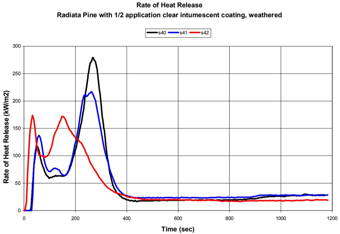
**Figure 12: Heat Release Rate – System I**
