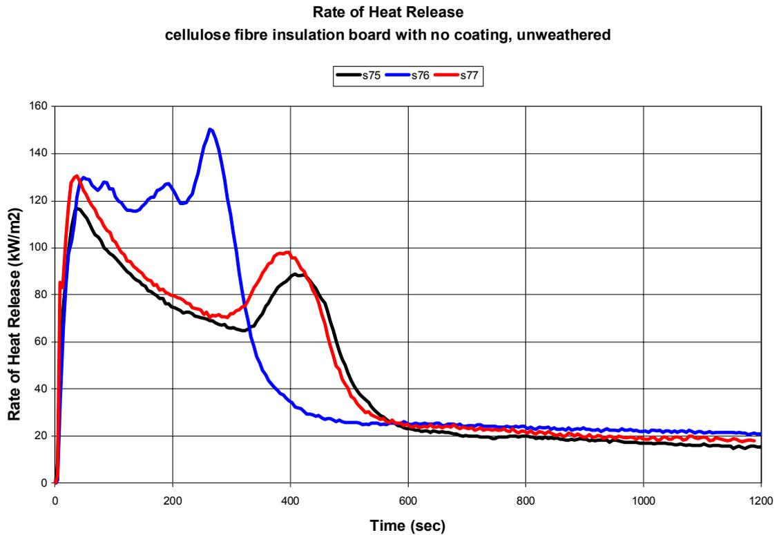
**Figure 19: Heat Release Rate – System S**
