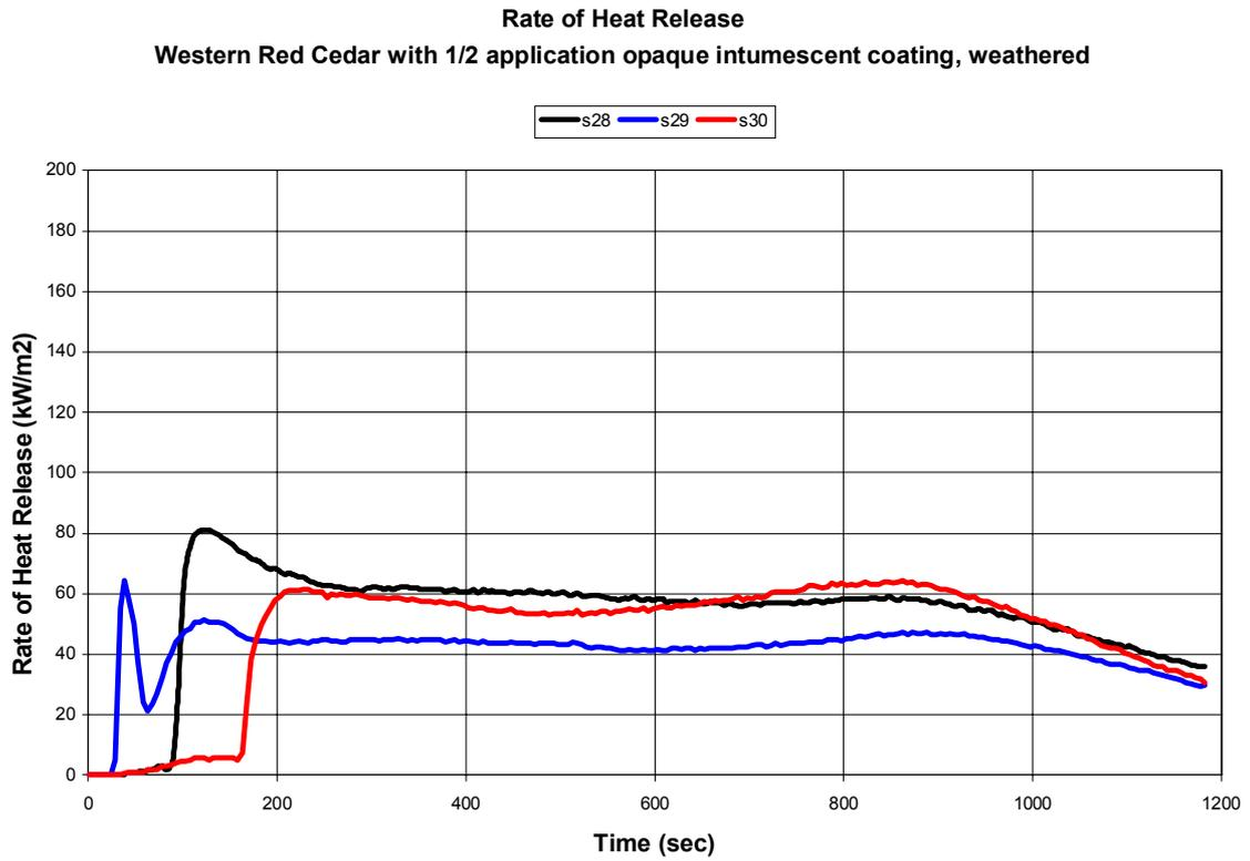
**Figure 22: Heat Release Rate – System O**
