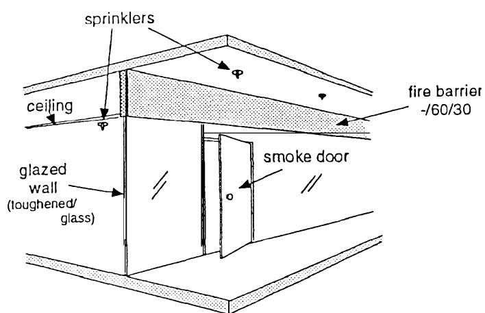
FIGURE 8.2 BOUNDING WALL CONSTRUCTION
