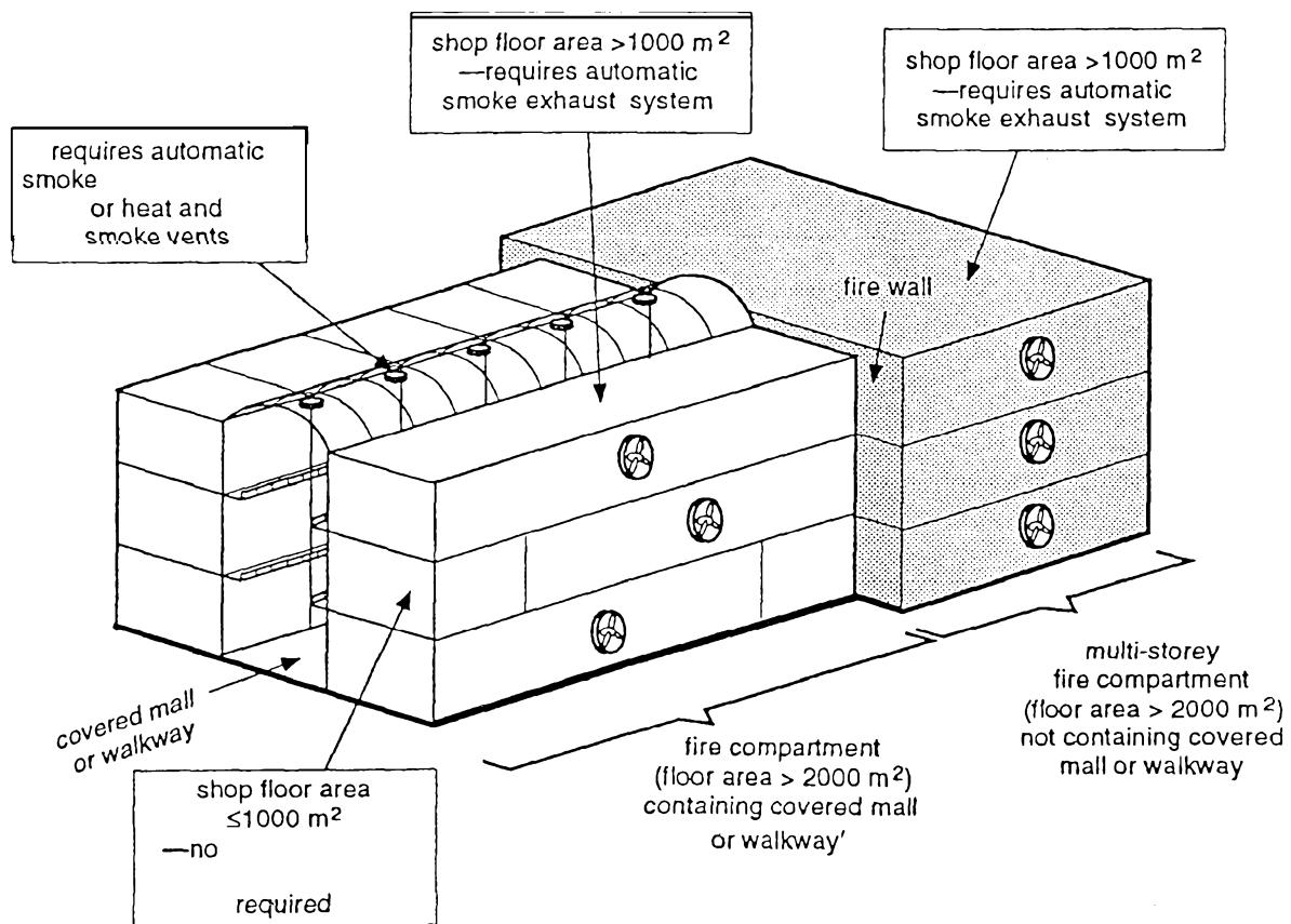
FIGURE 7.3 SPRINKLERED THREE STOREY BUILDING
