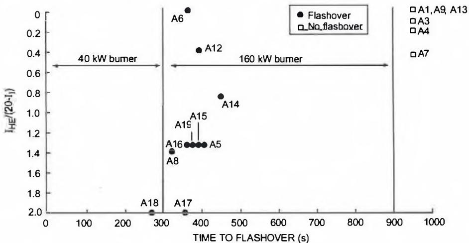
Figure F3 – Comparison of a relationship based on Early Fire Hazard Test Ignitability Index and Heat Evolved Index with time to flashover in the ASTM Room Fire Test
