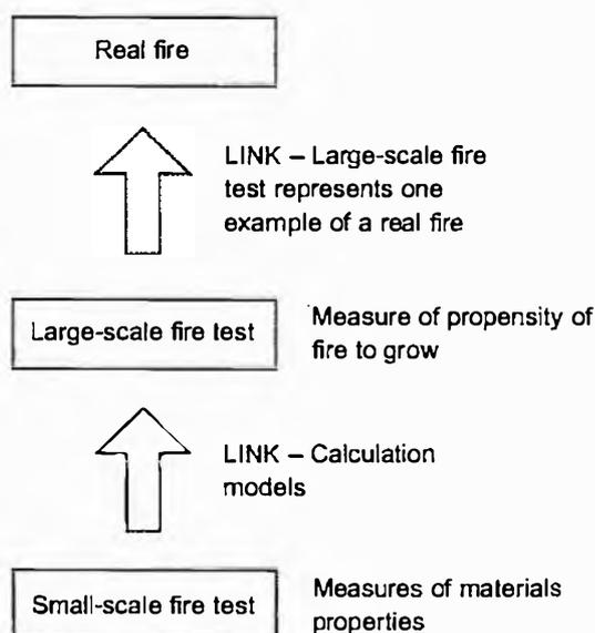
Figure 6.1 – Relationship between fire tests and real fires
