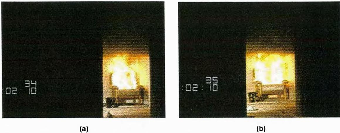
Figure 9.2 – Burning armchair in ISO room after 130 s: (a) plasterboard walls and ceiling; and (b) lauan plywood walls and plasterboard ceiling
