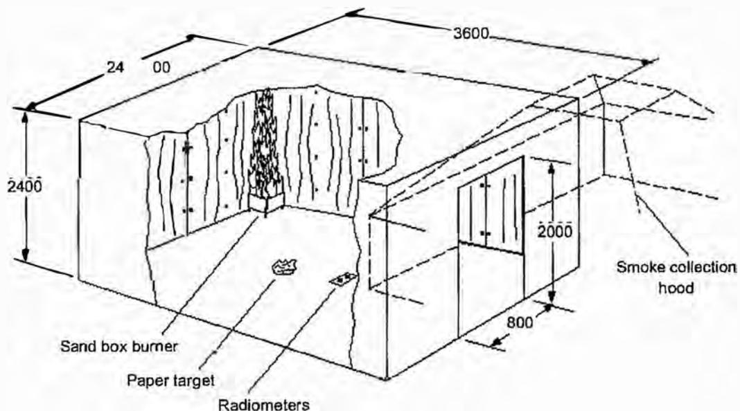
Figure 6.2 – Room fire test
