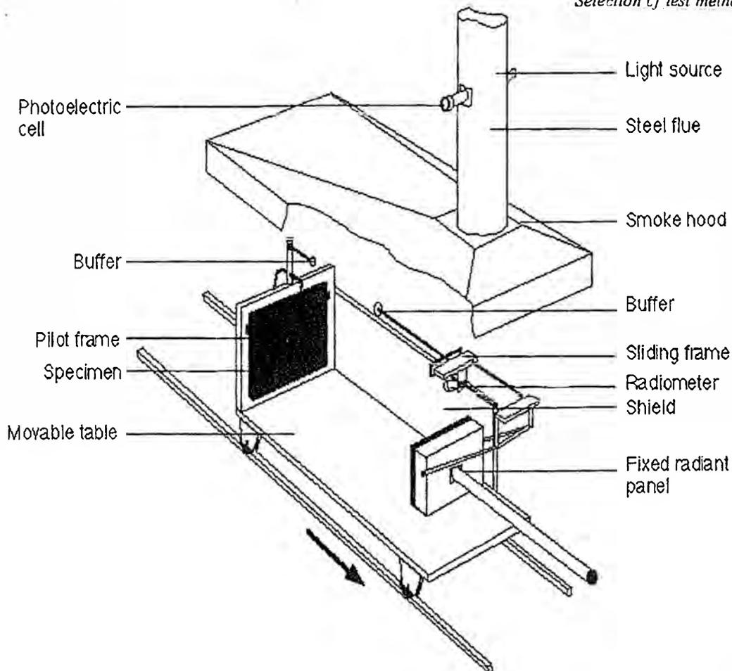
Figure 6.5 – Early Fire Hazard Test
