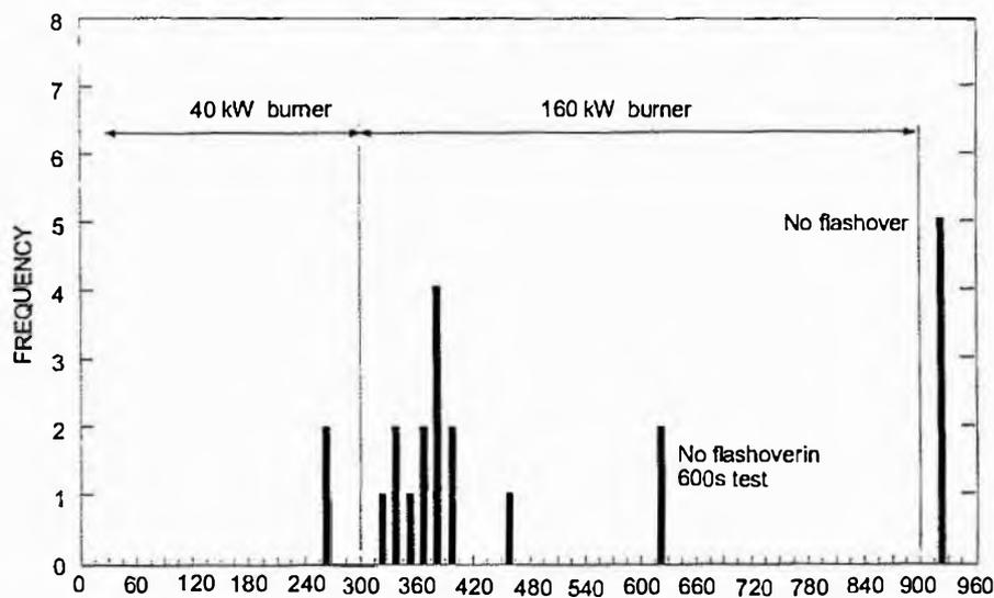
Figure 7.3 – Distribution of occurrence of flashover in the ASTM Room Fire Test
