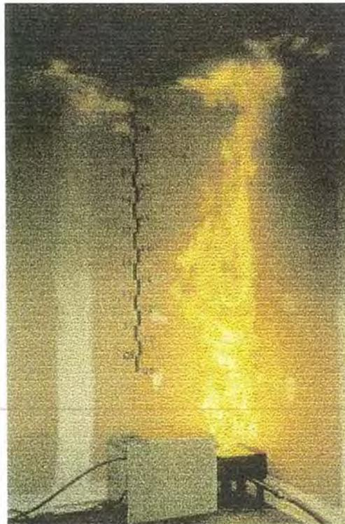
Figure 6.4 – Illustration of a 300 kW ignition source (2.7 m ceiling)
