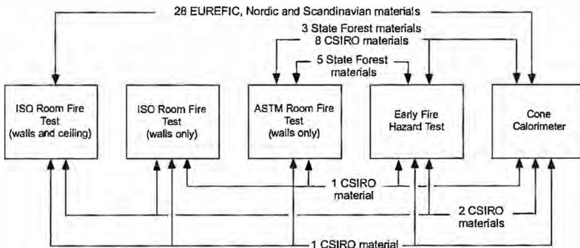
Figure 7.4 – Data available for comparing fire tests
