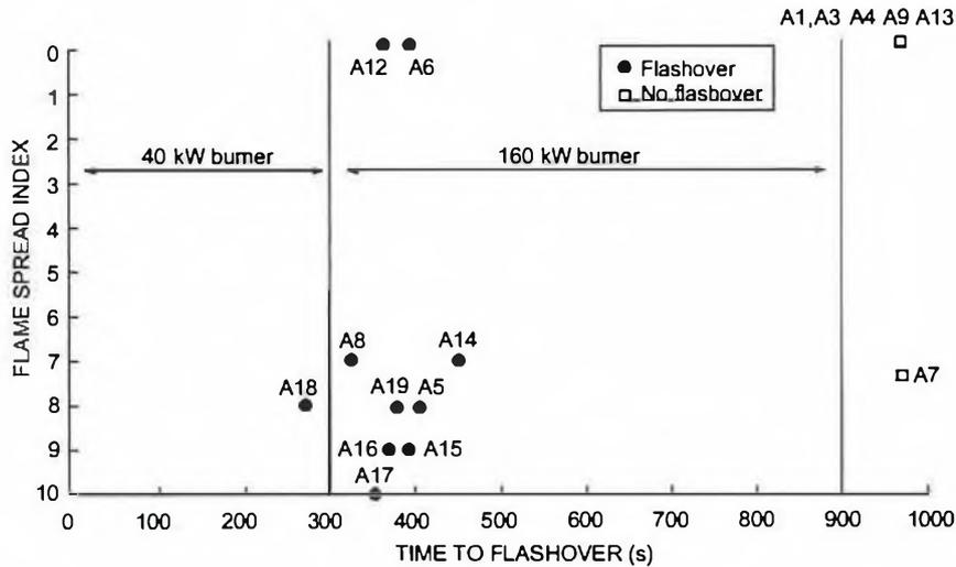
Figure F1 – Comparison of Early Fire Hazard Test Flame Spread Index with time to flashover in the ASTM Room Fire Test
