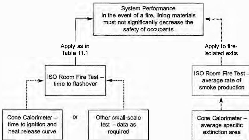
Figure 11.1 – Proposed control system for wall and ceiling linings
