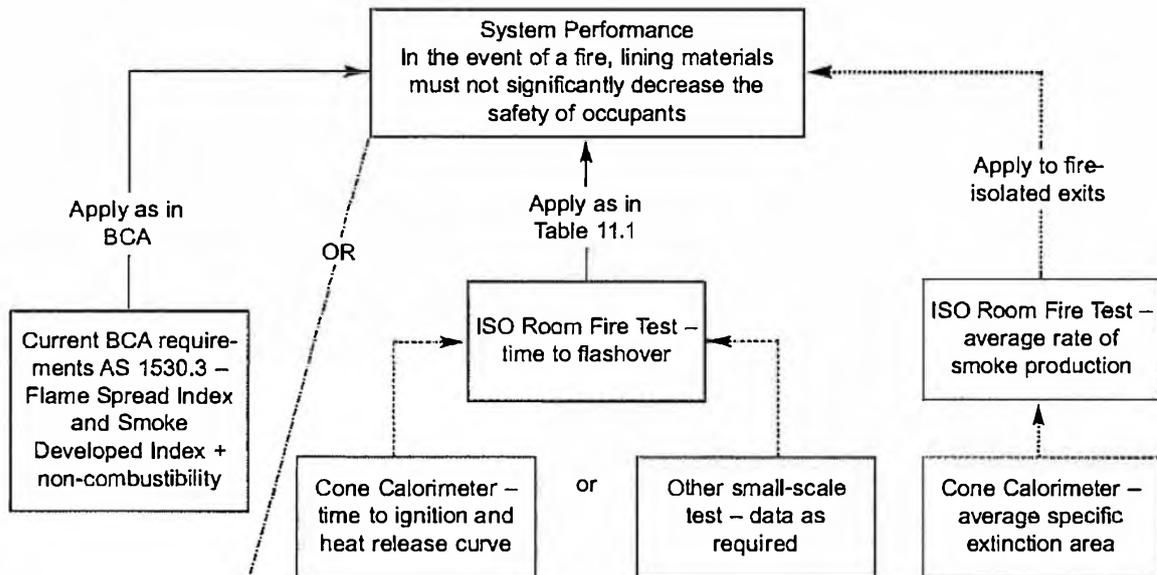
Figure 11.2 – Proposed parallel control system for wall and ceiling linings
