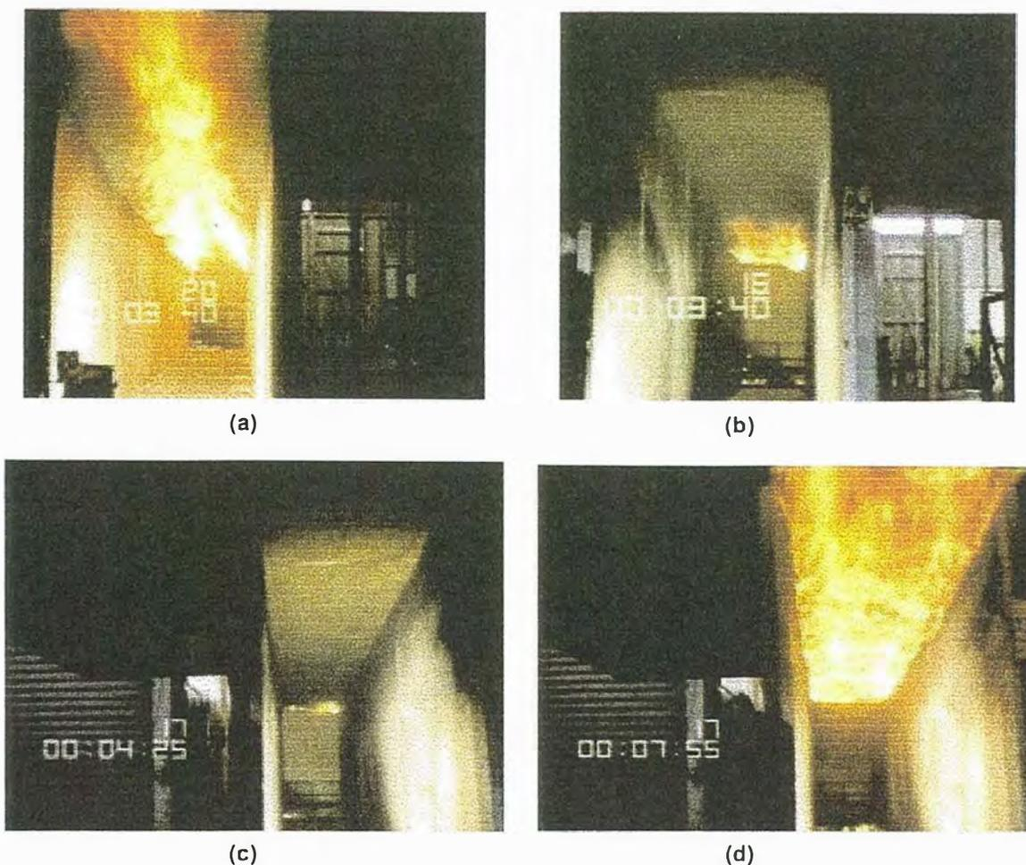
**Figure 7.1 – Flame spread in an experimental corridor following a flashover fire in an adjoining room: (a) lauan plywood walls; (b) lauan plywood ceiling; (c) treated hoop pine plywood walls; and (d) treated hoop pine plywood ceiling**
