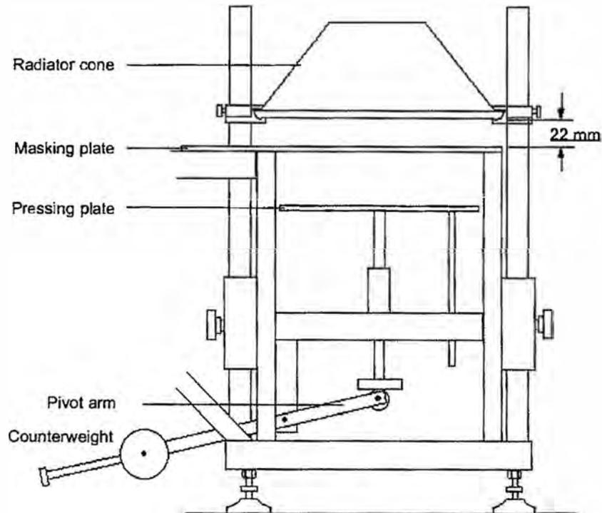
Figure 6.7 – ISO ignitability apparatus
