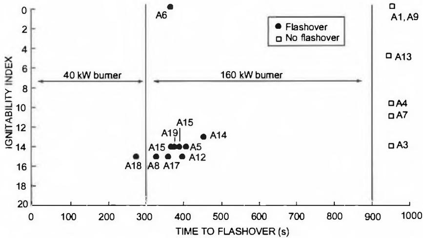
Figure F2 – Comparison of Early Fire Hazard Test Ignitability Index with time to flashover in the ASTM Room Fire Test
