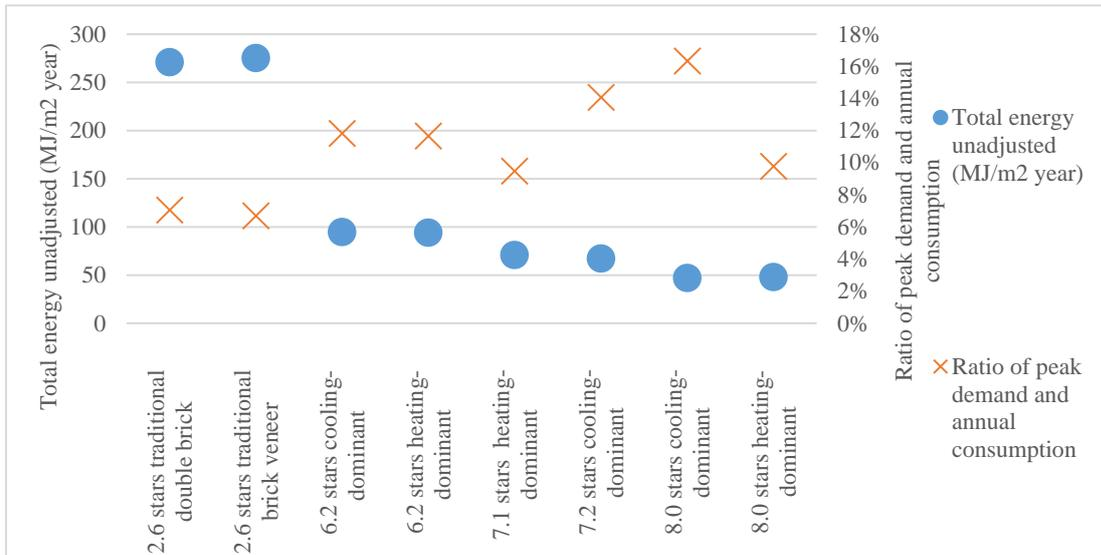
Figure 8 Ratio of peak cooling demand and annual energy consumption of the design scenarios in Adelaide
