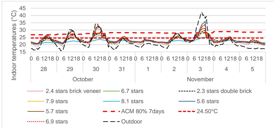
Figure 13 Overheating analysis of a north-facing bedroom during a medium heatwave period in Sydney
