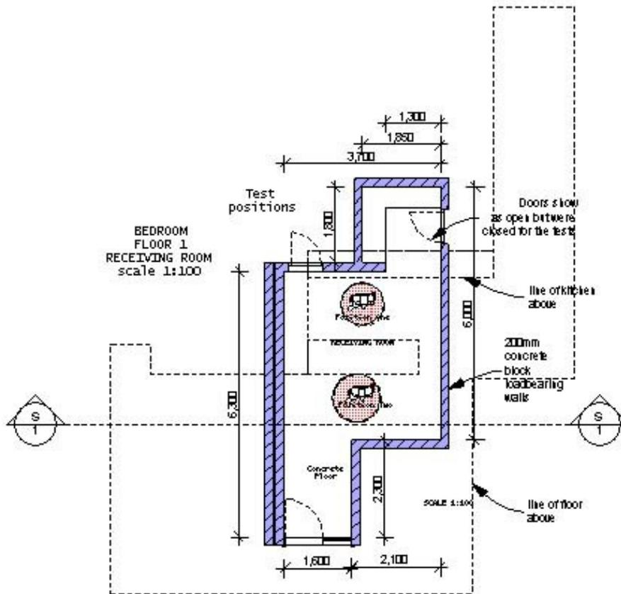
**FIGURE 16 - FLOOR PLAN – BEDROOM FIRST FLOOR – RECEIVING ROOM**
