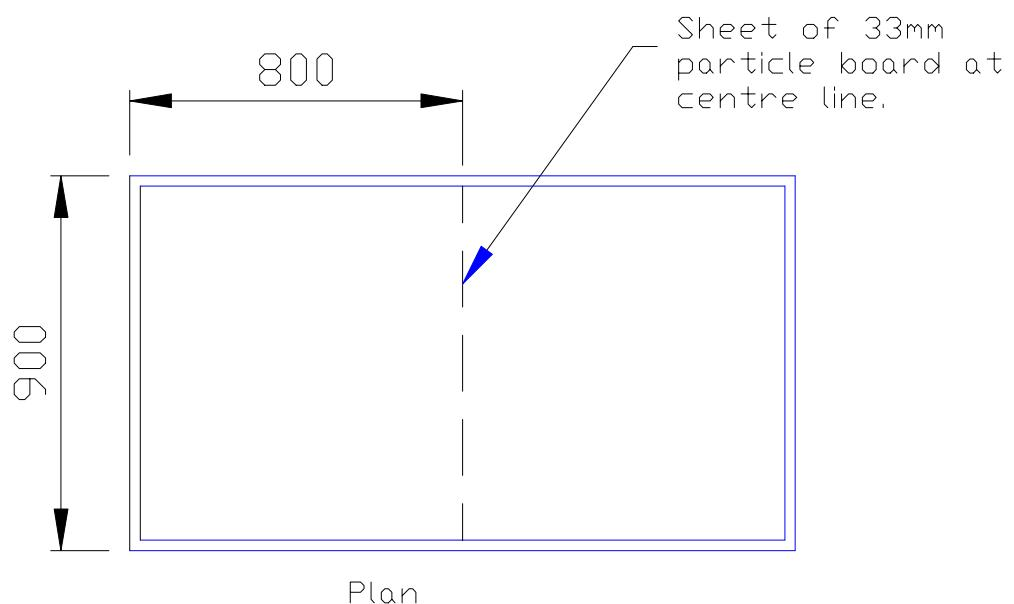
The top, one long side ( $1600 \times 700$ ), and one narrow side ( $900 \times 700$ ) located furthest from Bookcase #1, are to be lined with 33mm particle board. A  $900\text{mm} \times 700\text{mm}$  sheet of 33mm particle board is also to be fitted vertically at the centre line of the desk.
