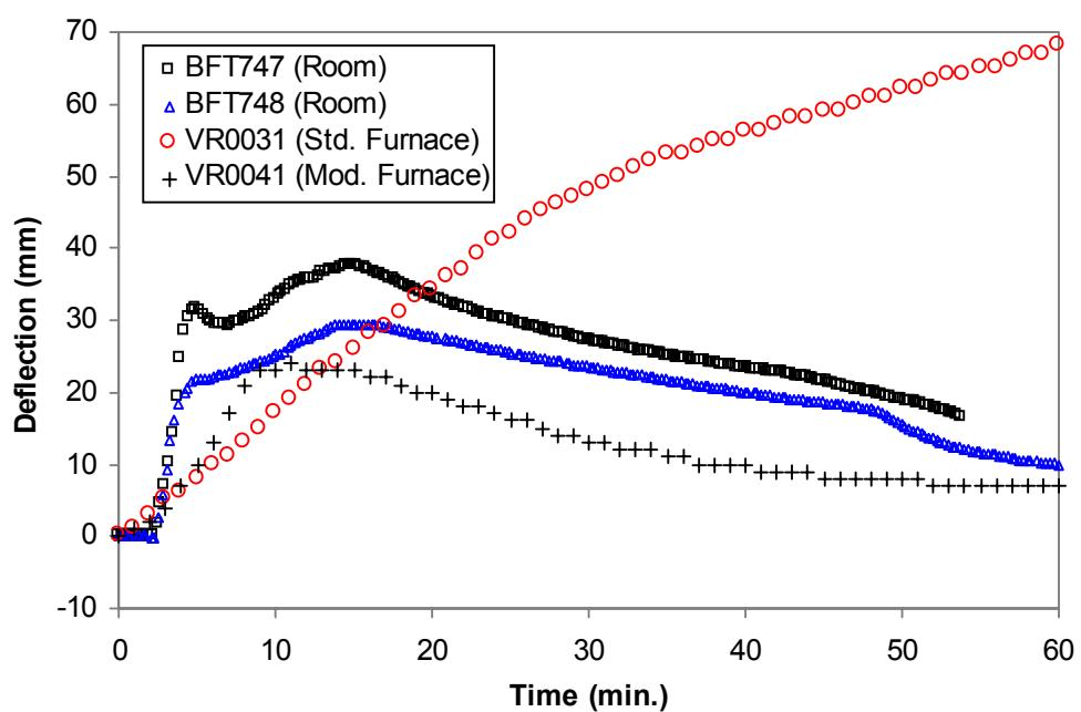
**Figure 6-3.** Modified furnace test on masonry wall: Comparison of deflection at mid-point of wall obtained during the furnace and room tests.
