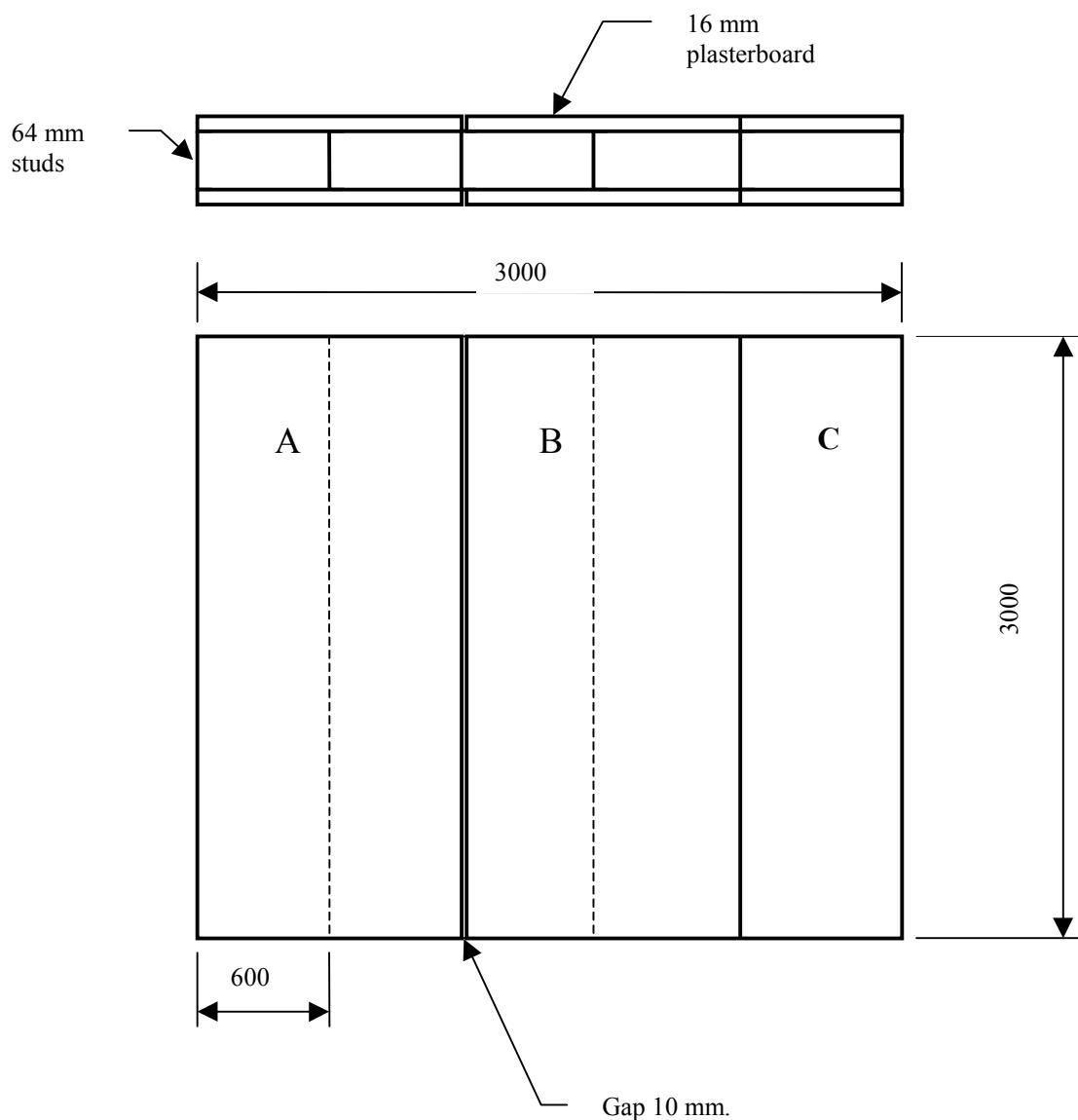
**Figure 1 Bad-workmanship plasterboard specimen wall.**
