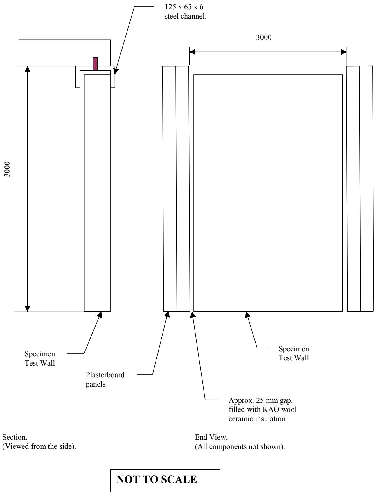
**Figure 2 Corner and joint specification for masonry specimen wall.**
