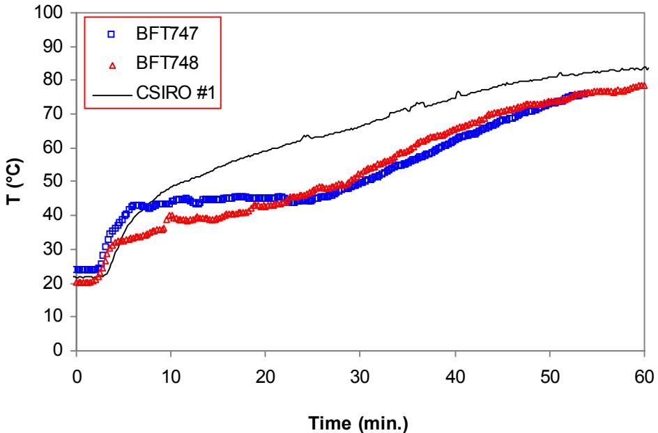
**Figure 4-10.** Masonry test walls: Unexposed-face average temperatures (thermocouples *U1-U7*) recorded during room tests.
