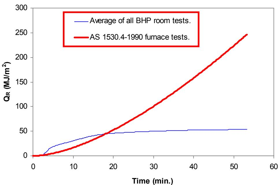
**Figure 7-2.** Values of  $Q_R$  evaluated near the exposed faces of the test walls.
