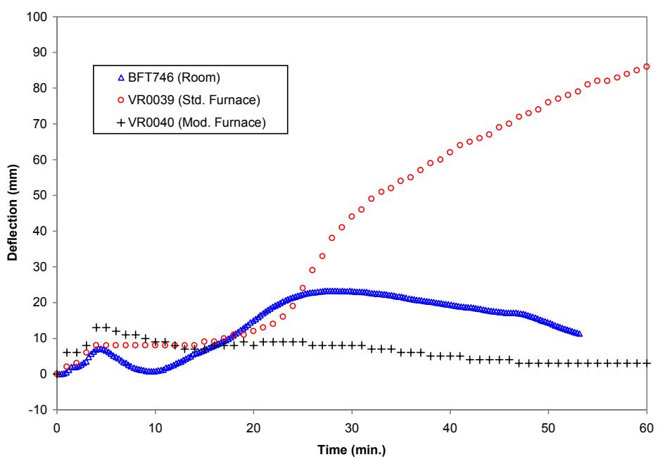
**Figure 6-6.** Modified furnace test on plasterboard wall: Comparison of deflection at mid-point of wall obtained during the furnace and room tests.
