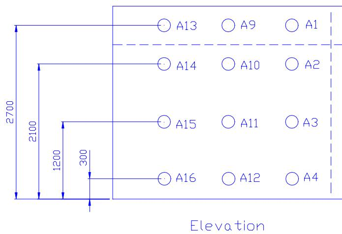
**Figure 3-3.** Location of air-temperature thermocouples.
