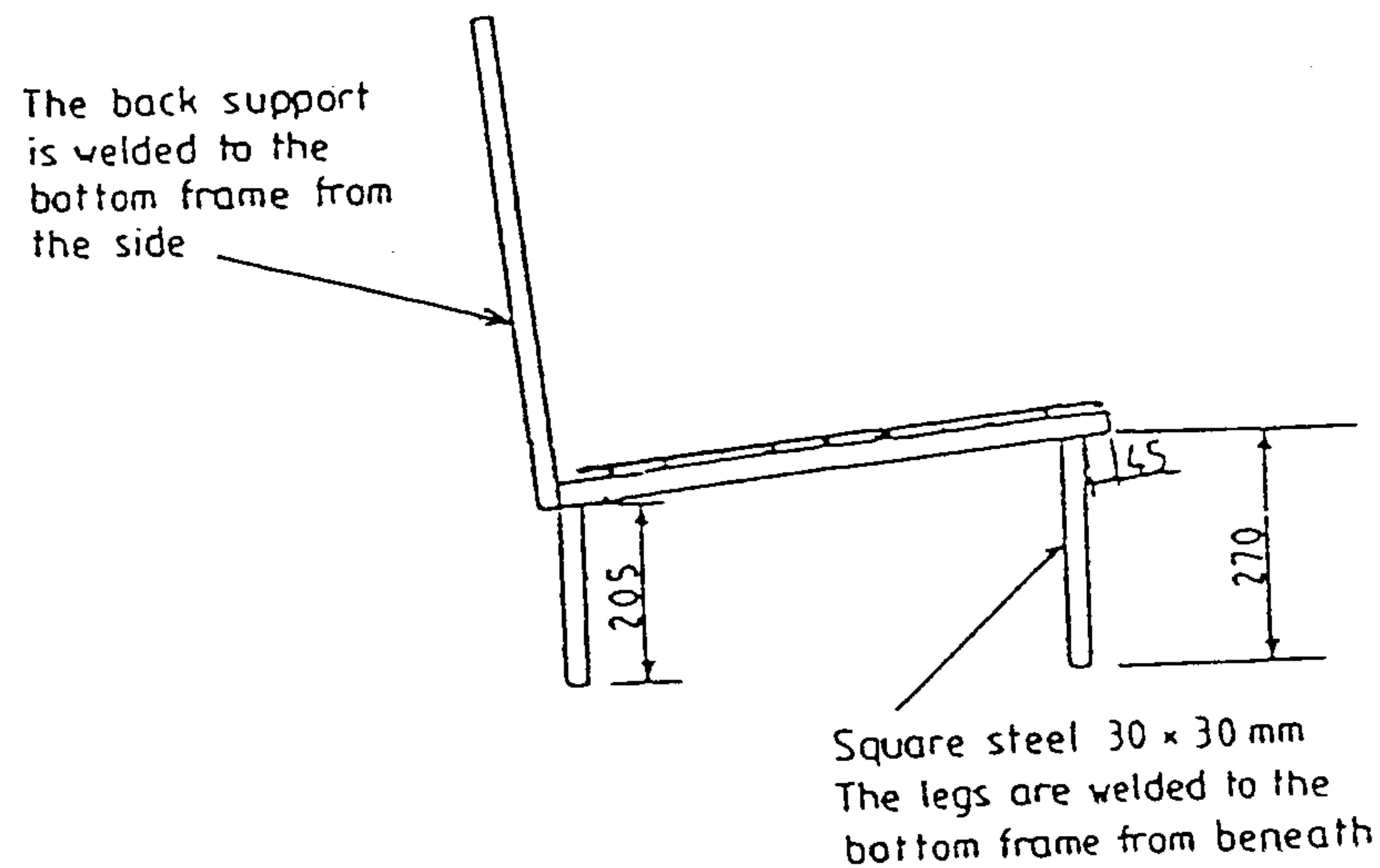
c) Side view of assembled seat frame.
