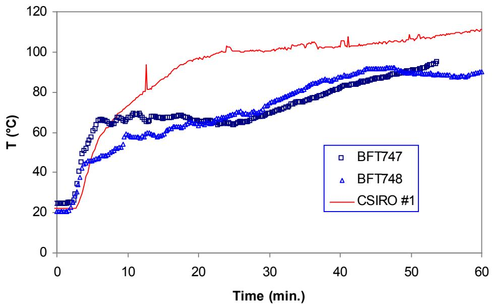
**Figure 4-11.** Masonry test walls: Unexposed-face maximum temperatures (thermocouples  $U1-U7$ ) recorded during room tests.
