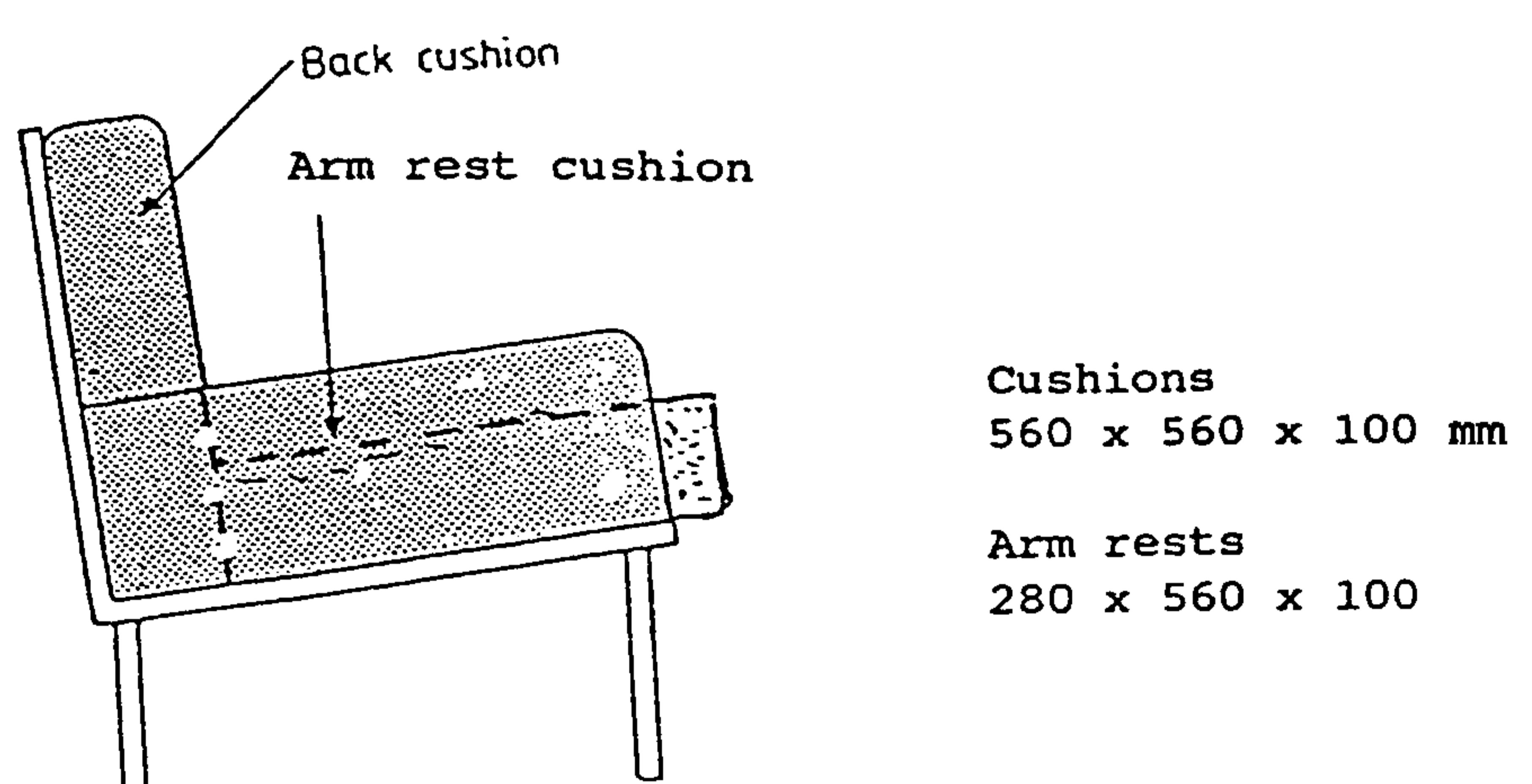
b) Side view (the arm rest of the steel frame not shown).
