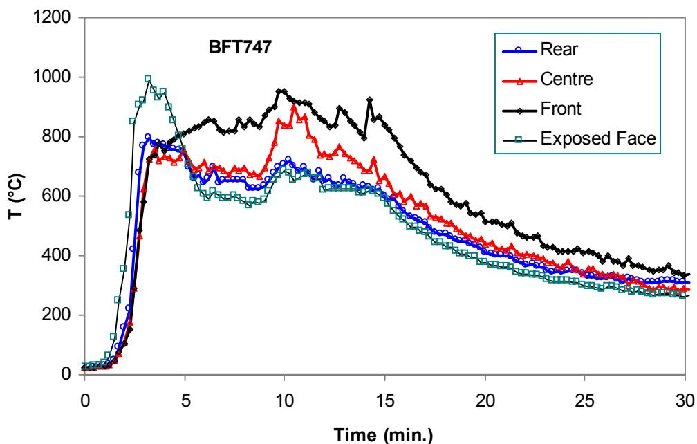
**Figure 4-3.** Temperature variations between front and rear of room.
