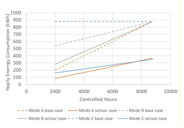
Figure 19. Comparison of energy use for Mode A, B and C cases of bathroom operation based on 100W load under sensor control. Note that in the Mode C base case, lights are always on.
