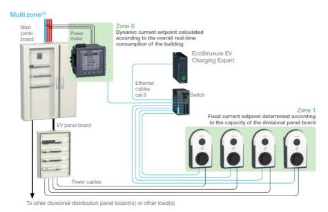
Figure 4: Active Load Management System<sup>2</sup>
