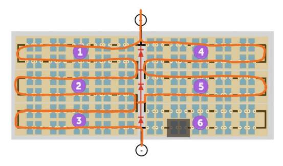
Figure 29: Half Cut Solar PV Panel Shading Response
