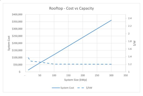
Figure 9: Cost vs Capacity for Rooftop Solar PV Installations
