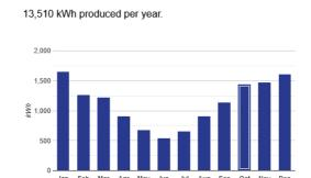
Figure 30 - Flat-panel installation @ 10kW North Facing (Sydney)
