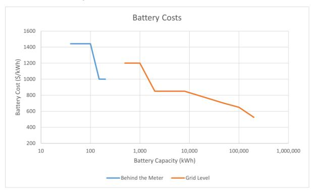
Figure 17: Battery Cost Behind the Meter and Grid Level Expressed as \$/kWh
