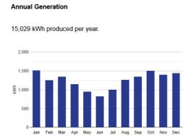
Figure 31 - Optimum angle tilt installation @ 10kW North Facing (Sydney)
