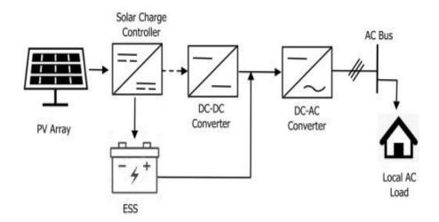
Figure 1: Solar PV system connected to load.<sup>24</sup>
