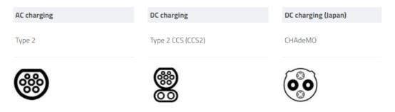
Figure 1: EV Charger Socket Outlet Types
