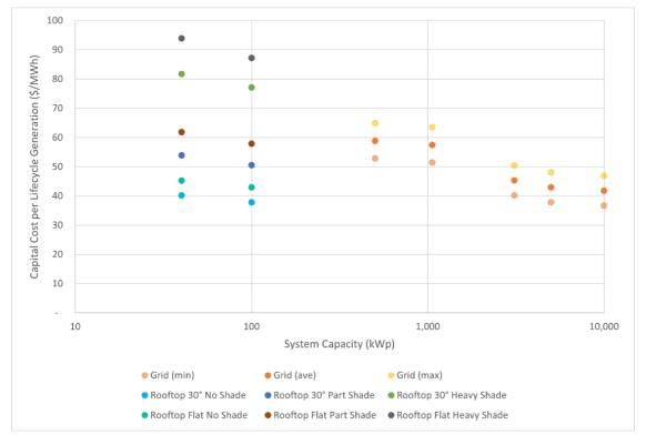
Figure 11: System Capital Cost per MWh of Lifecycle Generation for Rooftop and Grid PV
