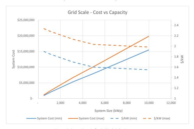
Figure 10: Cost vs Capacity for Grid Scale Solar PV systems
