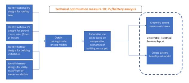
Figure 8. Outline methodology for the PV/Battery analysis
