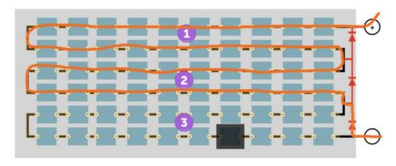
Figure 27: Conventional Solar PV Panel Shading Response<sup>26</sup>
