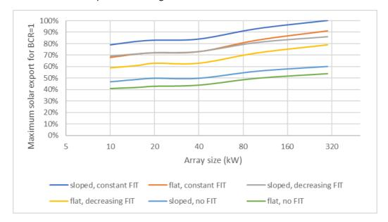
Figure 12. Maximum solar export from PV arrays for a benefit cost ratio of 1 under a range of Feed-in-tariff (FIT) scenarios, for sloped and flat installations.
