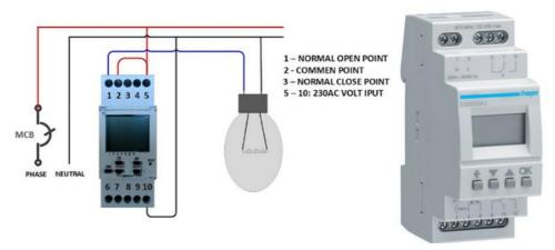
Figure 34: LCS-02 - Time switch operation
