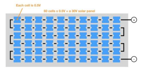
Figure 26: Conventional Solar PV Panel<sup>25</sup>
