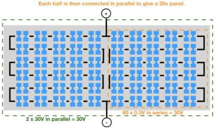
Figure 28: Half Cut Solar PV Panel<sup>27</sup>
